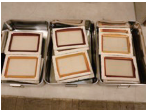
図3 比較のため数分～数時間のパターンで人工海水に浸す Fig. 3 For comparison, soaking in artificial seawater was performed in different styles for a duration of a few minutes to a few hours.
