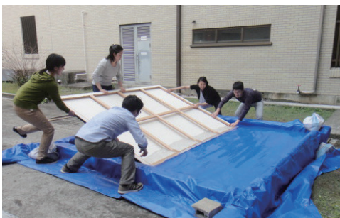
図5 被災作品と同寸のサンプルを人工海水に浸水させる Fig. 5 Soaking a sample that was the same size as the disaster-damaged artwork in artificial seawater.
