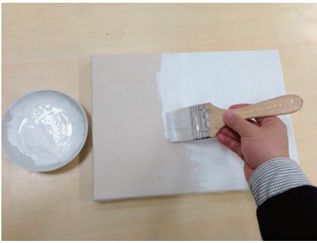
図1 キャンバス用綿布を木枠に張り込み、アクリル絵具を塗ってサンプルを作る Fig. 1 Samples were made by mounting cotton cloth on wooden frames and painting with acrylics.
