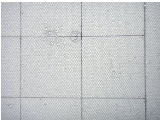
図6 浸水後、200号の同寸サンプルに縮みはみられない Fig. 6 No shrinking was observed in the identical sample after soaking.
